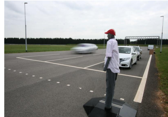
TRL Pedestrian detection target tested at InnovITS Advance test facility at MIRA UK.
