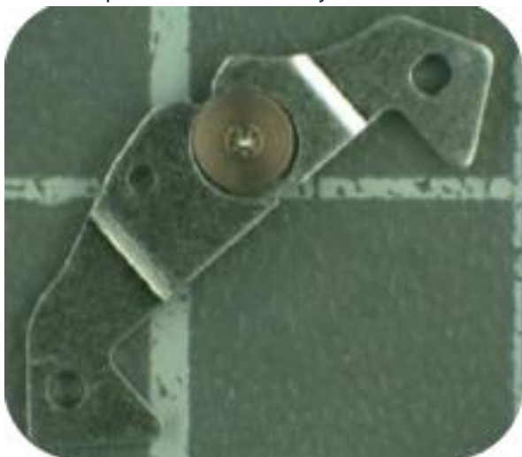
Figure 1b: rotor and stator of seiko mini-generator
