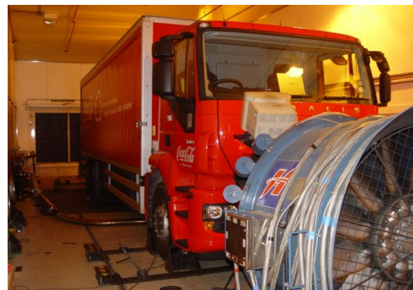
Figure 4 – The gas truck on the chassis dynamometer at Millbrook
